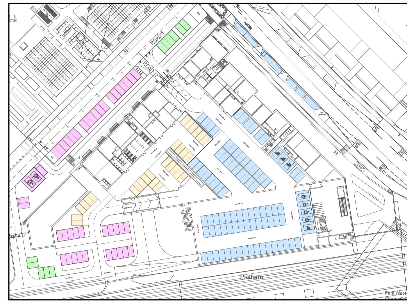
INSERT A HIGH DENSITY ON STREET/LOWER GROUND FLOOR LEVEL PARKING SPACE LAYOUT SCALE 1:1000
